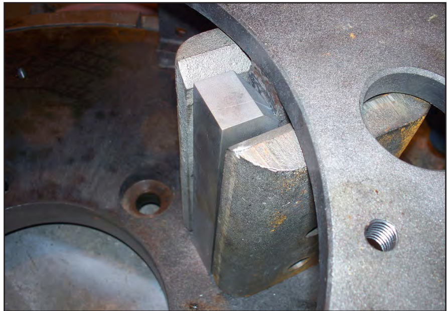
Inner Cap Showing Carbide Tip Installed
