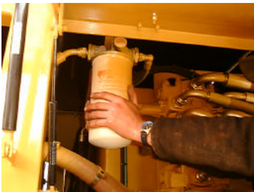
4:- Replacing hydraulic water trap
