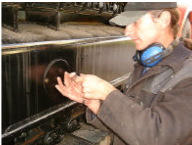
1:- Remove access cover from side of track
