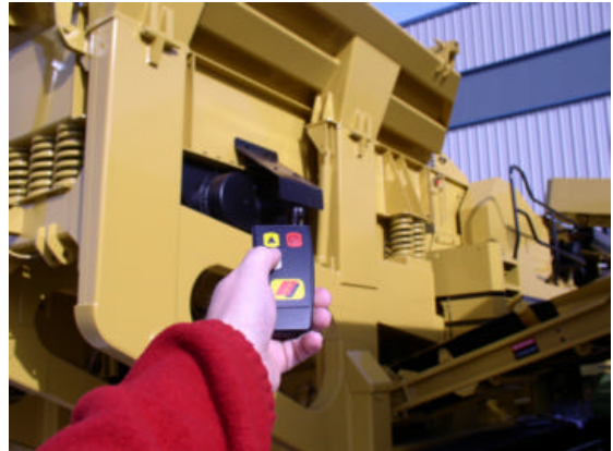
Starting/Stopping feeder speed using remote control.
