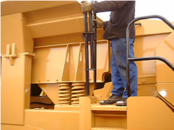
13a:- Locate safety gate in holes in RH side walkway.
