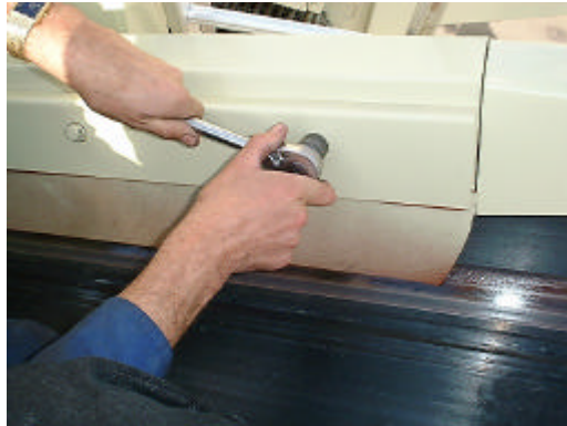
3:- Refit clamp fixing screws
