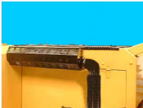
x) Machine is transported with exhaust stack in a lowered position. Release exhaust clamp & rotate stack to a vertical position. Re-tighten clamp.
