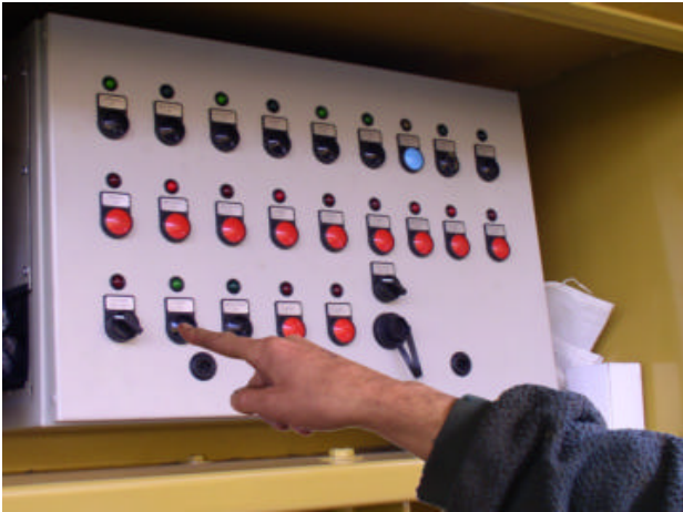
1:- Press button "Clamp On"
