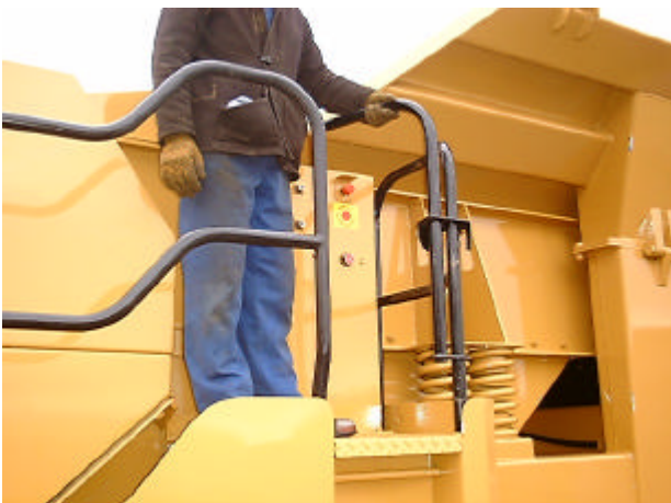
13c:- Raise up rotating gate section. (NOTE:- while operator is using the platforms the safety gates MUST be closed).
