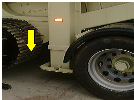
6:- Lower rear Jacking Legs to raise machine clear of the bogie locking mechanism .
