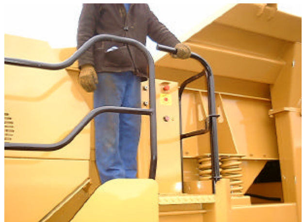
13d:- Rotate & lower gate into position. Repeat procedure on other side of machine.
