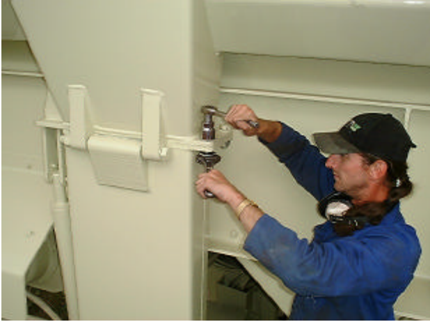
9:- Fit & tighten bolts at hopper leg/chassis. (Both sides)
