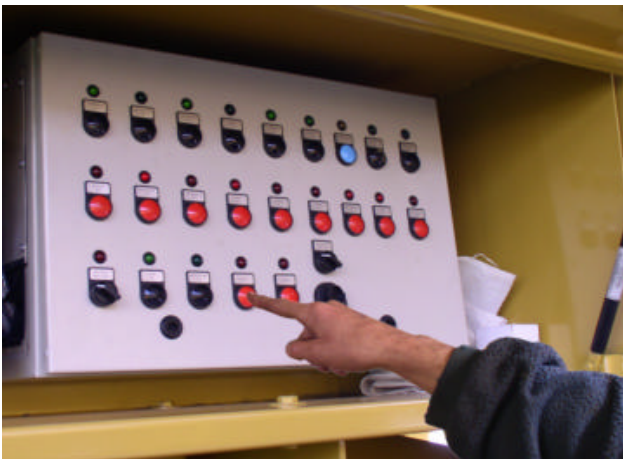
4b:- Press button "Jaw out" to open up Jaw.
