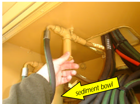
2:- Unscrew hand primer and pump up & down until a steady flow of fuel comes out of filters. (there must be no bubbles coming through fuel line). Re-secure hand primer after use.
