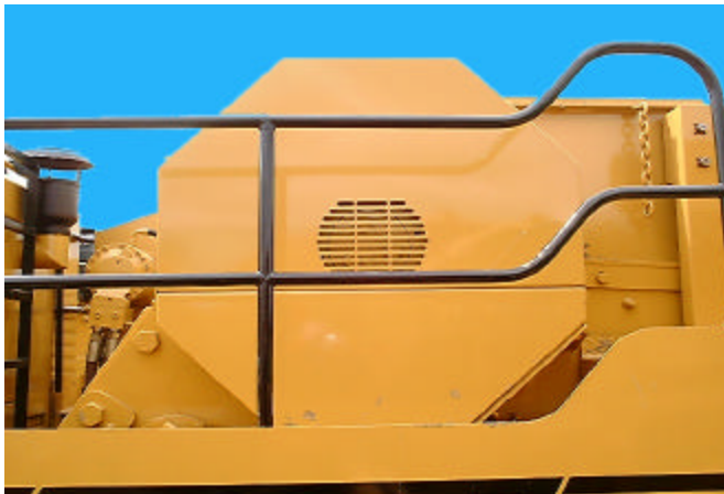
Look through slotted area on guard at alignment arrow on shaft end plate.
