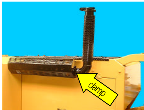
x) Machine is transported with exhaust stack in a lowered position. Release exhaust clamp & rotate stack to a vertical position. Re-tighten clamp.
