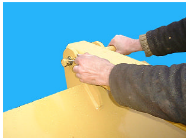
8:- Fit hopper cross-tie box & secure with pins & R-clip
