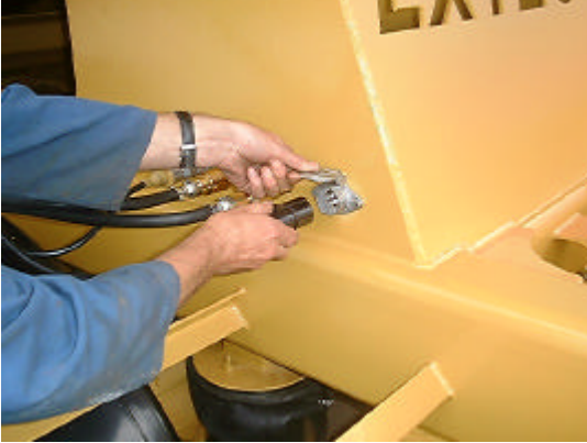
7:- Remove Bogie air brakes & lighting connections then tow away from machine.
