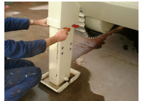
2:- Ensure that locking pins and R-clips are fitted BEFORE cleaning below machine
