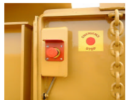
5:- Emergency stop on R/H side of crusher box.
