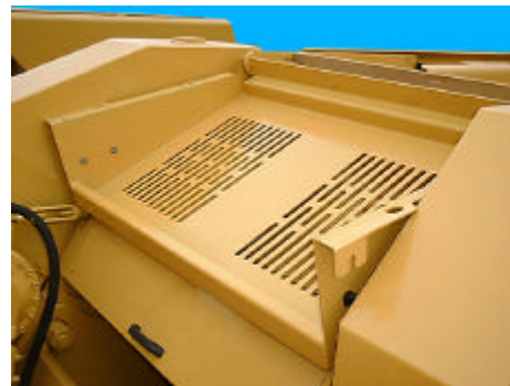
xi) Machine is transported with inlet chute cover in the open position.
