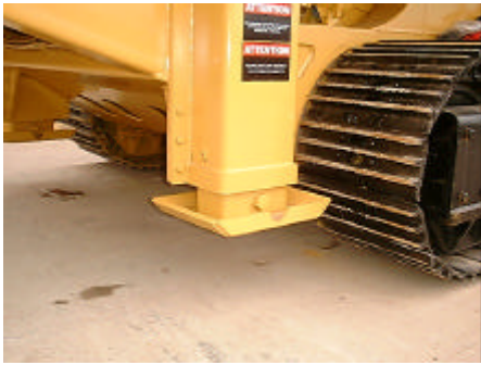
Jacking legs fully raised
