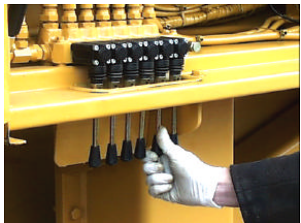
4b:- Activate levers to raise rear jacking legs
