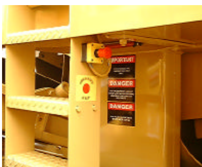
4:- Emergency stop on R/H side walkway ladder.
