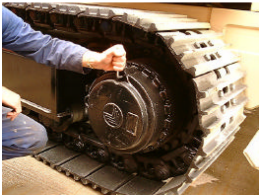
Removing filler plug
