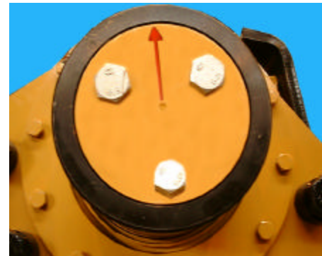
Alignment arrow points vertically up at minimum jaw opening.
