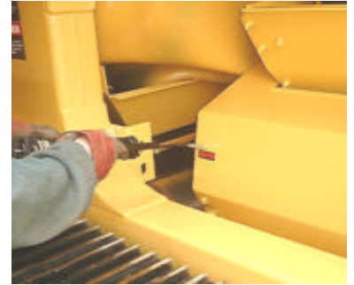
Side Conveyor lower bearings.
