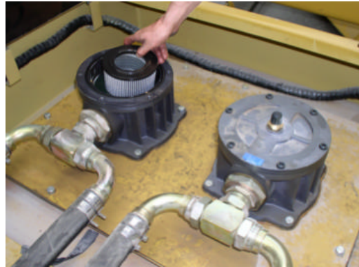
2:- Replace elements if service indicator is red
