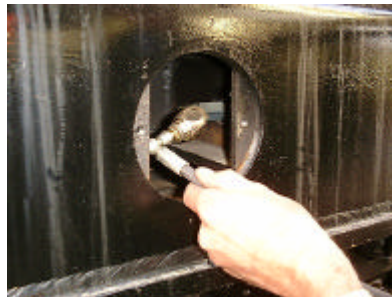
2:- Fit grease adapter to grease point inside tracks
