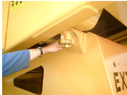
4:- Unlock bogie from machine (4 positions).
