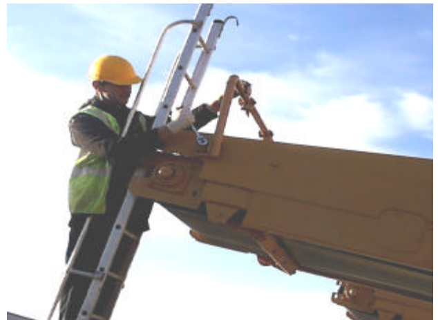
12b:- Fix main conv. spray bar in working position.
