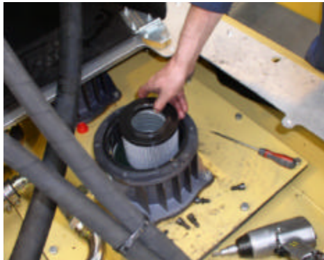
2:- Replace element if service indicator is red
