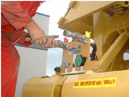
3:- Remove tractor unit air brakes & lighting connections then unhitch from machine.
