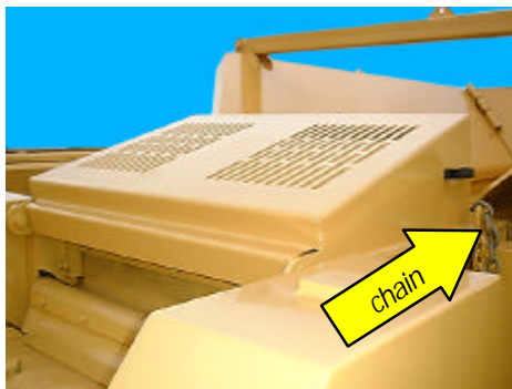
xi) Rotate cover into position & attach chains.
