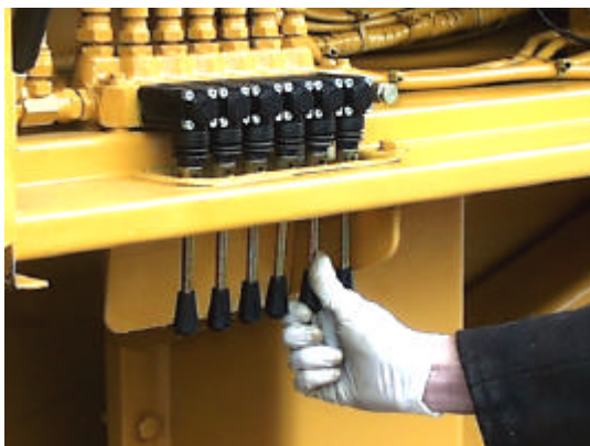
5:- Rear Jacking Legs lever.
