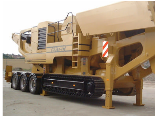
2:- Lower front Jacking Legs to raise fifth wheel neck by approximately 100 mm.
