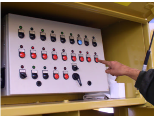
3:- Press button "main conveyor lower"
