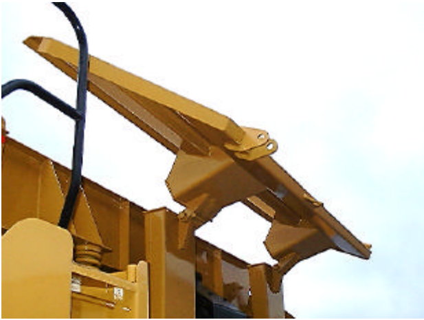
Hopper side being raised
