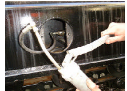
3:- Pump grease into tracks until they are tight.
