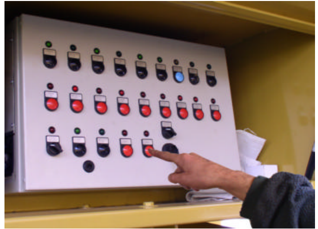
4a:- Press button "Jaw in" to close up Jaw.
