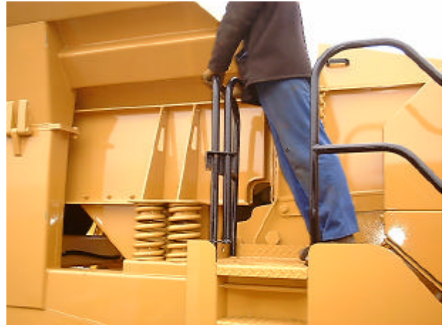
13b:- Push safety gate firmly down into holes.
