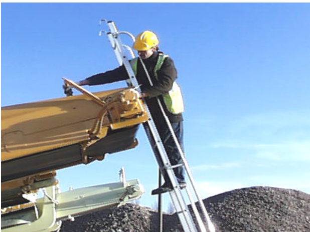
12a:- Raise main conv. spray bar to working position.
