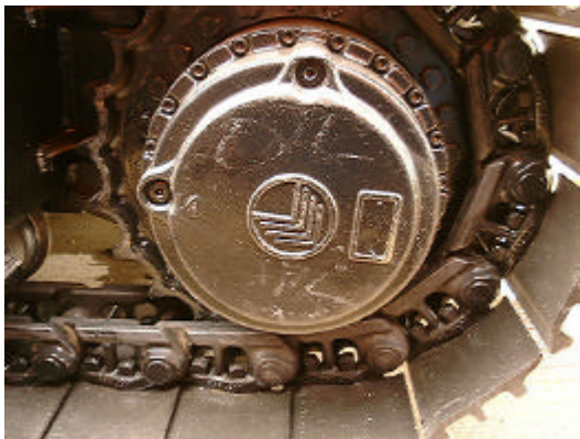
Track gearbox in correct position to refill motor with oil.
