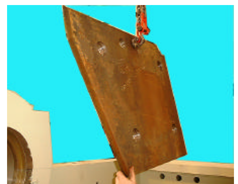
6:- Fit new jaw plate, ensuring that all debris is cleaned from location slots.
