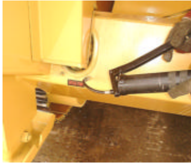
Main Conveyor lower bearings
