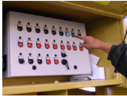
5:- Press button "Tracks On"
