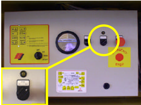
1:- Turn engine speed switch to position No.2
