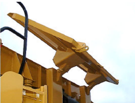
Hopper side being raised
