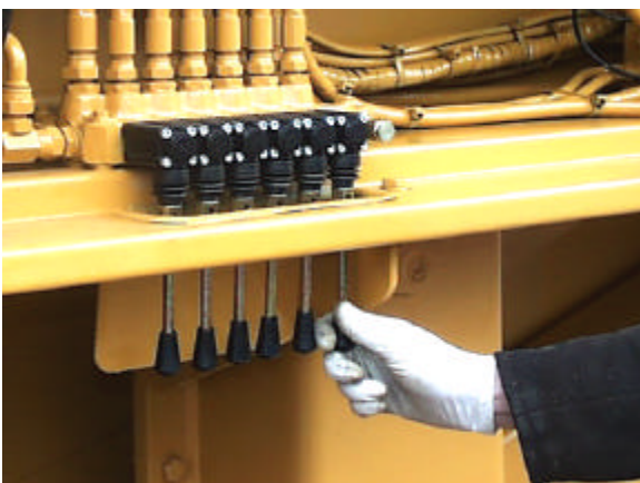
4a:- Activate levers to raise front jacking legs
