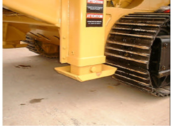
8:- Retract both front and rear jacking legs so that weight of machine is taken on tracks .
