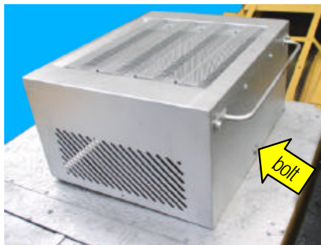
xii) IF FITTED - Machine is transported with oil cooler in the down position. Release transportation bolt & rotate oil cooler into position. Remove transport bracket then attach cover plate to deck & retain oil cooler with stay bar.
