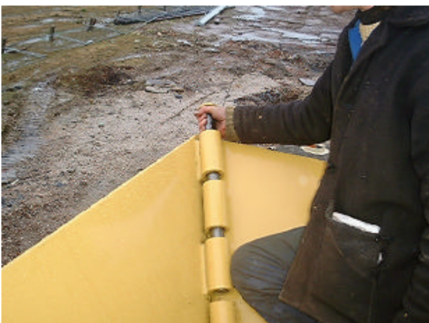
7:- Fit locking pins to hopper sides/rear
