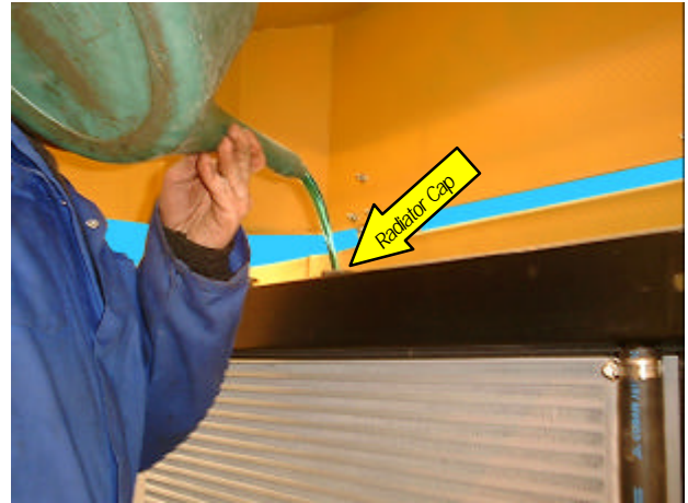
Check radiator water level & refill if necessary.
